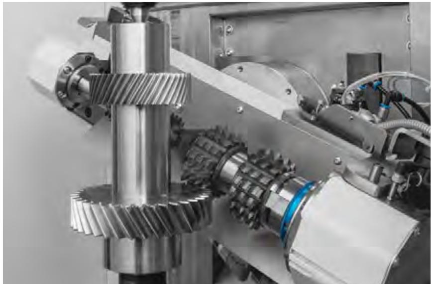
An optional Chamfer Hob head with outboard support accepts up to four Chamfer Hobs for two gears on a shaft or for non-standard gears.
