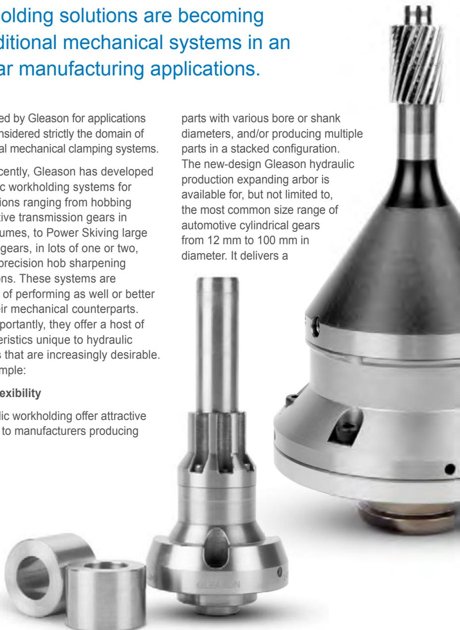
very powerful and consistent clamping force when hydraulic fluid pressure is applied to a thin-walled expansion sleeve, precision-machined out of tough tool steel. The sleeve expands as required by the application uniformly over its entire chucking length. This gives a single arbor the inherent flexibility to meet the requirements of a variety of parts with different bore diameters.
