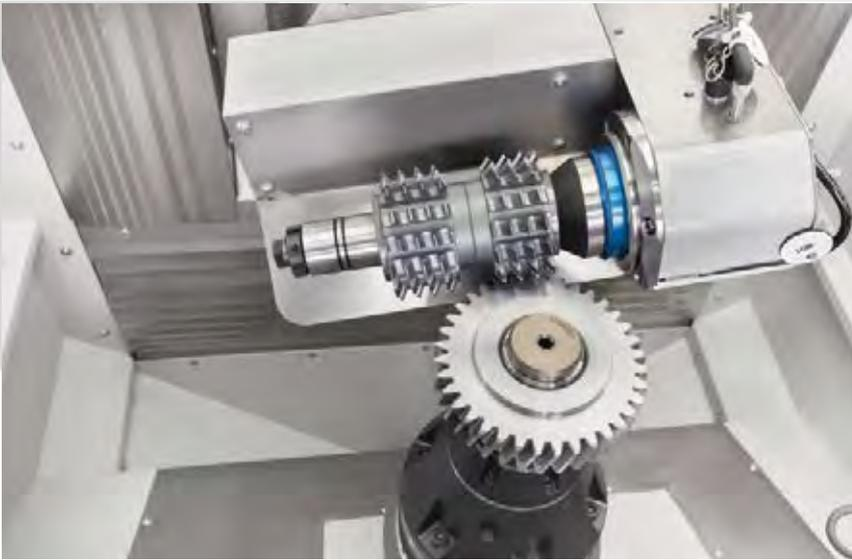
The new Chamfer Hobbing process offers an extremely efficient solution to create the desired chamfer without considerable secondary burrs.
