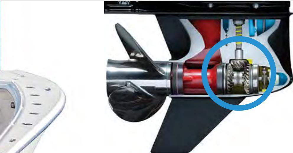
Mercury Marine applies new Gleason manufacturing and inspection technologies to produce the quiet, reliable bevel gears and pinions that help propel a new generation of high-horsepower outboards.
