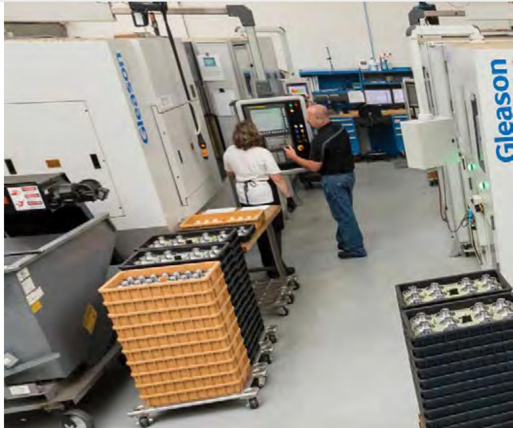
Four Gleason 280Cs now do the work of some 40 manual machines, cutting part changeover time from a complete shift to around an hour.
