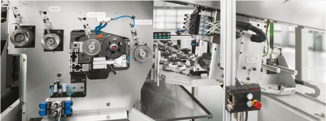
The new simplified automation concept serves both disc-type parts and shafts. One linear loading axis transports parts from the conveyor directly to the workpiece spindle. Roll checking of workpieces is executed in between part pickup station and loading onto the workpiece spindle. The diamond master dressing gear and dressing roll are both stored and brought into action with the same grippers that also transfer the workpieces.
