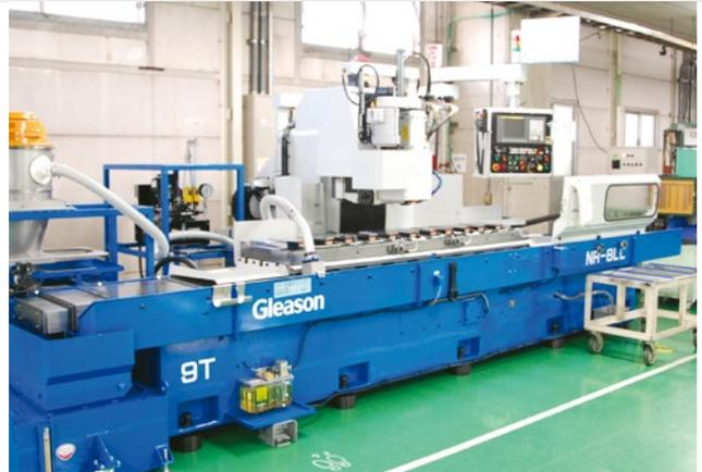
KHK relies on Gleason-Saikuni Rack Manufacturing technologies, both milling and grinding, to improve production of high-precision racks for important rack and pinion business.
