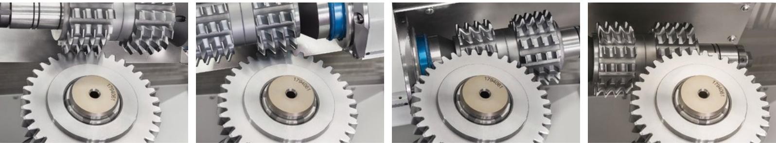
The new Chamfer Hobbing process offers an extremely efficient solution to create the desired chamfer without secondary burrs.
