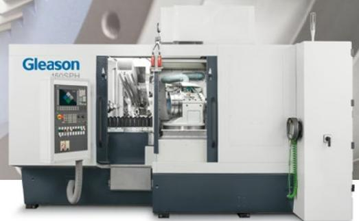
In the early 1990s, Gleason did a great deal of pioneering work to develop honing into an independent Power Honing process. In fact, today's machines facilitate removal rates which are in no way inferior to those of grinding.
