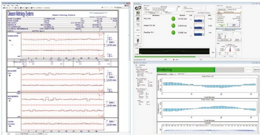
Non-contact (laser) index and profile inspection can be performed on all the gear teeth in a matter of just 10 to 15 seconds, as compared to several minutes when done conventionally.
