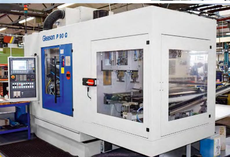
The P90G is capable of hobbing and grinding spur and helical gears and pinions up to module 3 mm and diameters up to 100 mm. It offers the user three different grinding methods to cover a wide range of applications:
