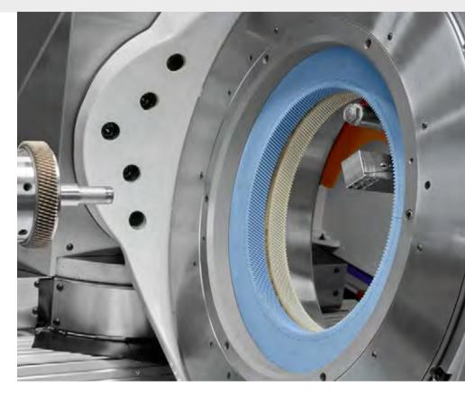
diamond dressing tools on the work spindle (Fig. 2). The location of the dressing tools ensures that the position of the teeth on the honing rings does not change either absolutely or relatively – even after dressing of the honing rings. Loading/unloading of dressing tools to the work spindle, as is often the case in other honing applications, cannot reliably achieve this important quality aspect.
