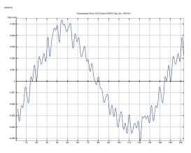
Figure 4: Transmission error of all teeth inspection
