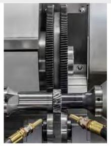
Chamfer rolling process is done in parallel to gear hobbing on the Gleason P90CD horizontal hobbing machine.
