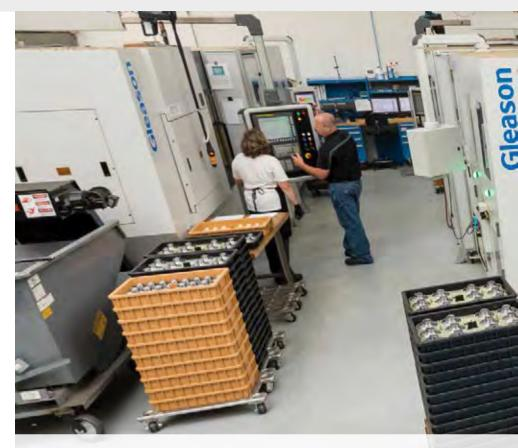
Four Gleason 280Cs now do the work of some 40 manual machines, cutting part changeover time from a complete shift to around an hour.
