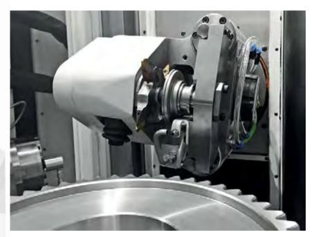
Contour Milling in parallel to gear hobbing on the Gleason 400HCD does not add cycle time and is ideal for truck-size gears.
