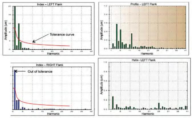
Figure 1: Fourier analysis of Index, Profile (Involute) and Helix (Lead).
