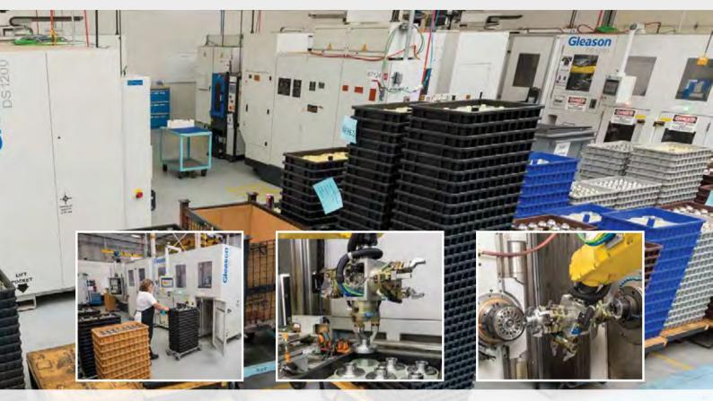
Each 280C has a Gleason DS1200 Machine Tool Loader, which uses a stackable tray system and robot to automate part load/unload. The automation uses less floor space, and puts more parts in-process, than conveyor systems.
