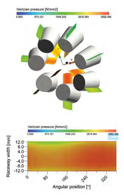
Figure 2: Bearing race surface stress calculation.
