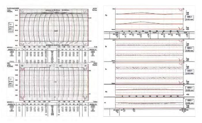
Figure 3: Quality of the larger gear on a stepped pinion, shown to be achieving DIN 5 or better.
