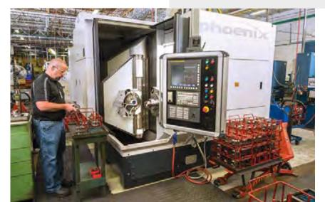
Mercury Marine has added significant new capacity to its finish grinding operations with a Gleason 280G, which also connects to GMS inspection via GEMS to automate the correction process.
