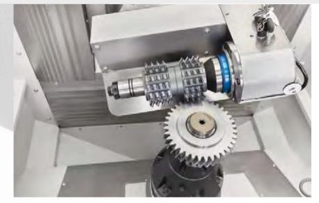
The new Chamfer Hobbing process offers an extremely efficient solution to create the desired chamfer without considerable secondary burrs.
