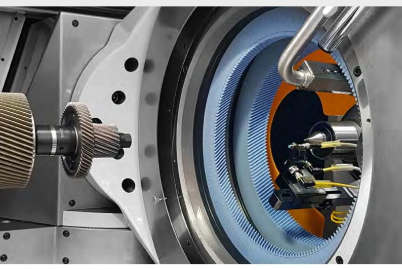
Figure 2: 260HMS can apply the Combi Honing process to produce stepped pinions reliably and at the quality levels needed to ensure the correct installation position in the planetary transmission. Integrated sensors measure the position of all teeth on both gear as well as the position of the index hole on the face side.
