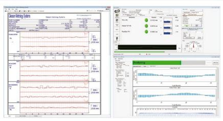
Non-contact (laser) index and profile inspection can be performed on all the gear teeth in a matter of just 10 to 15 seconds, as compared to several minutes when done conventionally.
