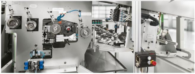
The new simplified automation concept serves both disc-type parts and shafts. One linear loading axis transports parts from the conveyor directly to the workpiece spindle. Roll checking of workpieces is executed in between part pickup station and loading onto the workpiece spindle. The diamond master dressing gear and dressing roll are both stored and brought into action with the same grippers that also transfer the workpieces.
