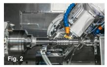
there is a whole range of Gleason Power Skiving machines, from the 300PS to the 600PS, which can be expanded to a diameter up to 800 mm.
