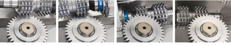
The new Chamfer Hobbing process offers an extremely efficient solution to create the desired chamfer without secondary burrs.
