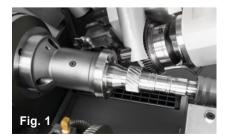
outstanding choice for machining both shafts (Figure 1) and internal gears. Furthermore, the 100PS can be equipped with an integrated chamfering/ deburring station for external gears. The chamfering process is interpolated before the final cut and helps achieve finished machining quality afterwards. For internal gears, the 100PS has a patented deburring unit which can be programmed via 2 NC axes. As a special feature, the machine provides the option for skiving worms (Figure 2).
