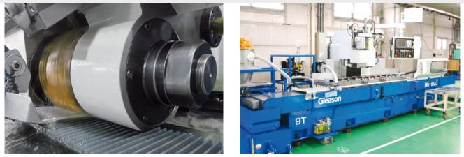
KHK relies on Gleason-Saikuni Rack Manufacturing technologies, both milling and grinding, to improve production of high-precision racks for important rack and pinion business.
