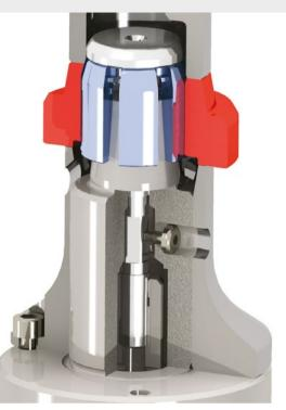
Segmented collets give workholding maximum wear life; with sizes and an expansion range covering the bore clamping requirements of the most common cylindrical – and some bevel – gear types and sizes.
