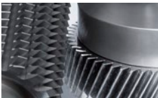
Hobbing with parallel chamfer cutting
