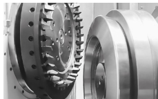
500C highly efficient production of bevel gears up to 500 mm in diameter.
