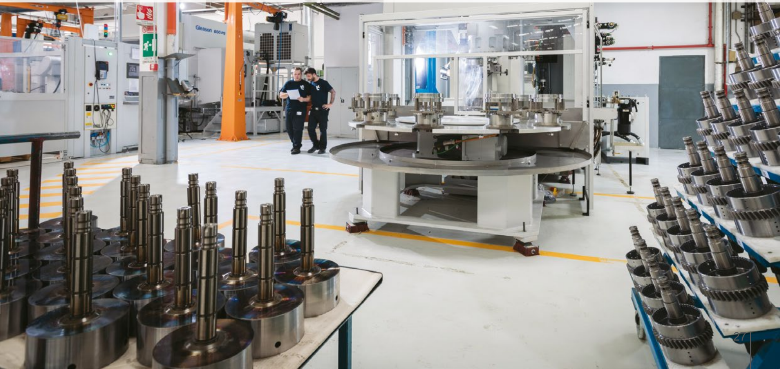
Three Gleason 600PS Power Skiving Machines have proven to be four to five times faster than their shaping machine predecessors, and improved quality by two DIN classes.
