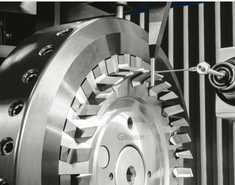
Figure 3: Automatic building and truing of Pentac®Mono with 500CB.
