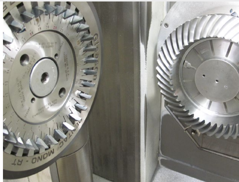
Figure 4: Phoenix 280CX after cutting with 7.5" Pentac®Mono-RT cutter head.
