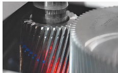
Combined double flank roll testing and laser scanning
