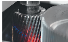
In-process gear inspection via roll testing and laser scanning.
