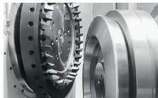
500C High volume production of medium-sized bevel gears.
