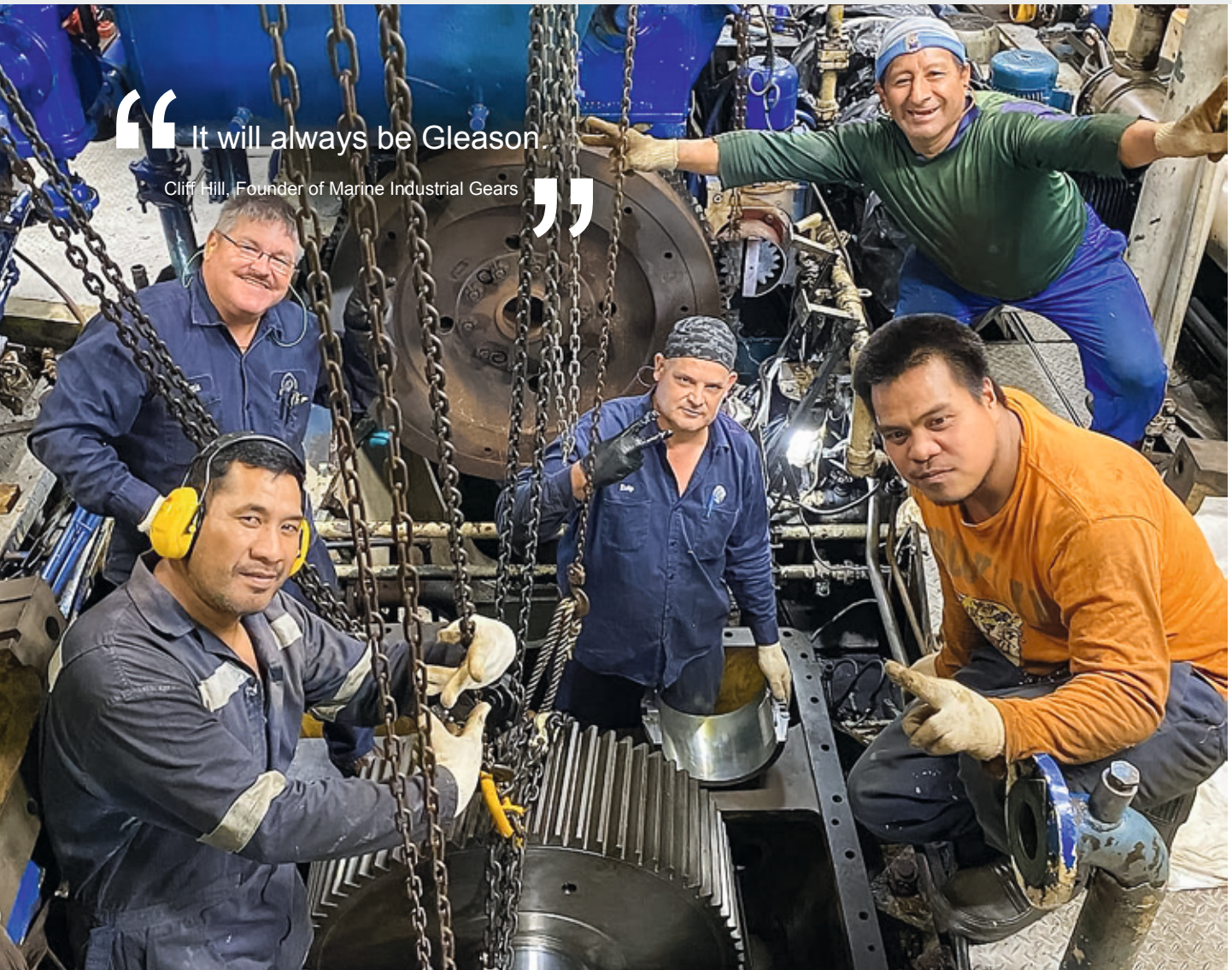
The MIG Crew “on board”, installing a new transmission gear on high seas.
