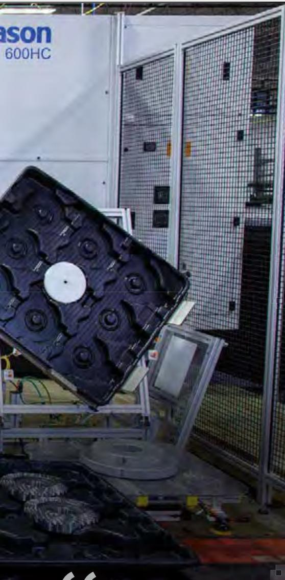
(Left) 2700AR in use at the SEW Eurodrive facility in Lyman, SC automates load/unload of larger bevel gears on a new Gleason 600HC Bevel Gear Cutting Machine, greatly reducing time and freeing up the operator for other tasks.
