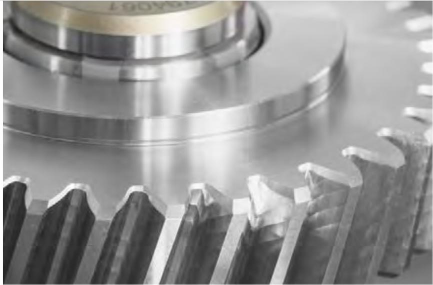
Chamfer Hobbing process can produce a variety of highly desirable chamfer forms. Unlike chamfer rolling, however, it does not generate a secondary burr requiring removal downstream.
