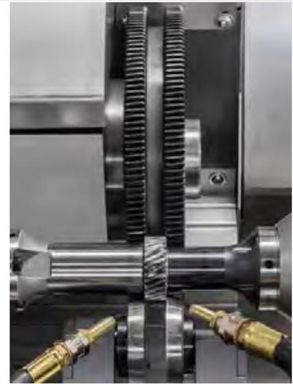
Chamfer rolling process is done in parallel to gear hobbing on the Gleason P90CD horizontal hobbing machine.
