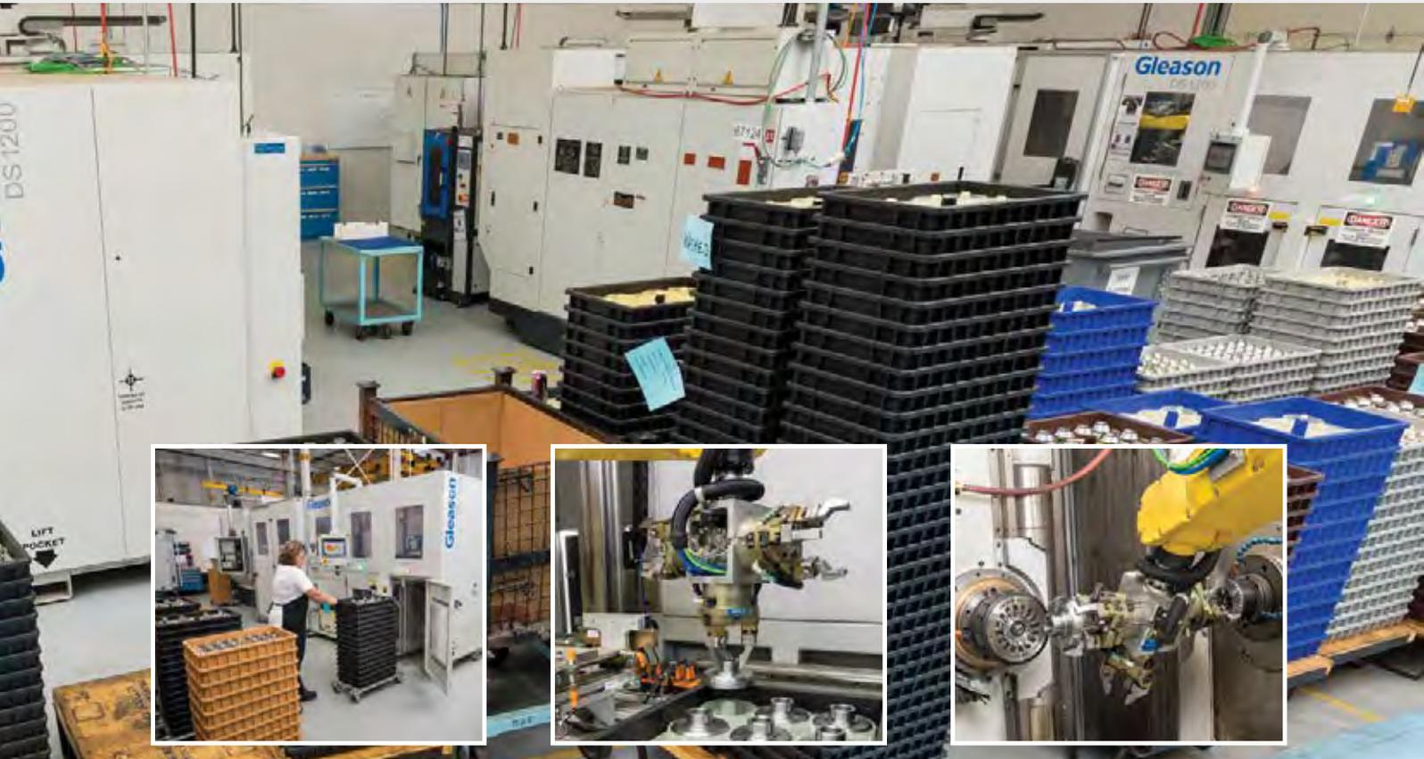
Each 280C has a Gleason DS1200 Machine Tool Loader, which uses a stackable tray system and robot to automate part load/unload. The automation uses less floor space, and puts more parts in-process, than conveyor systems.
