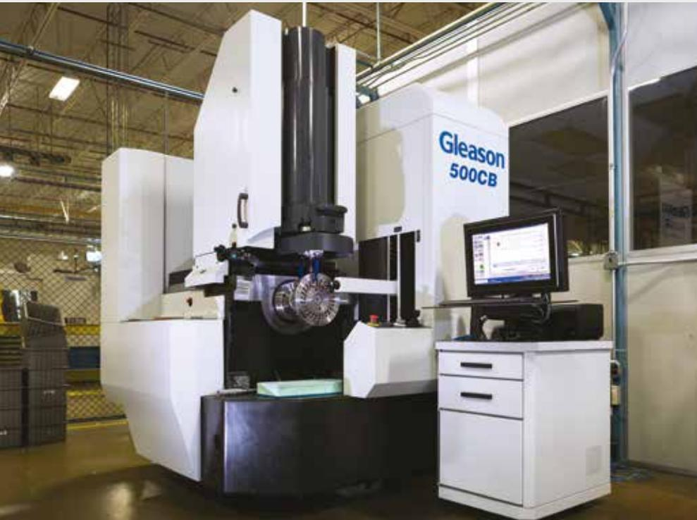
SEW Eurodrive was the Beta site for Gleason's first 500CB machine. Today, the machine is reducing cutter build times from the 90 minutes needed previously to less than 30 minutes.
