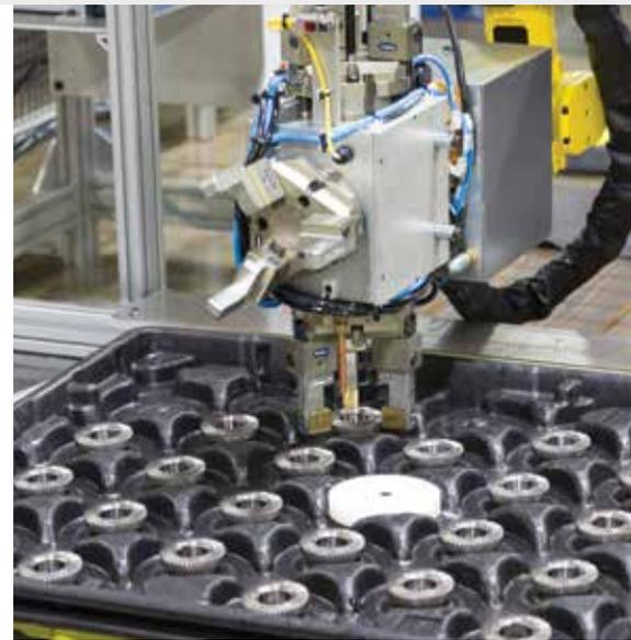
Load/unload automation is easily integrated with the 280G, further reducing non-productive time.
