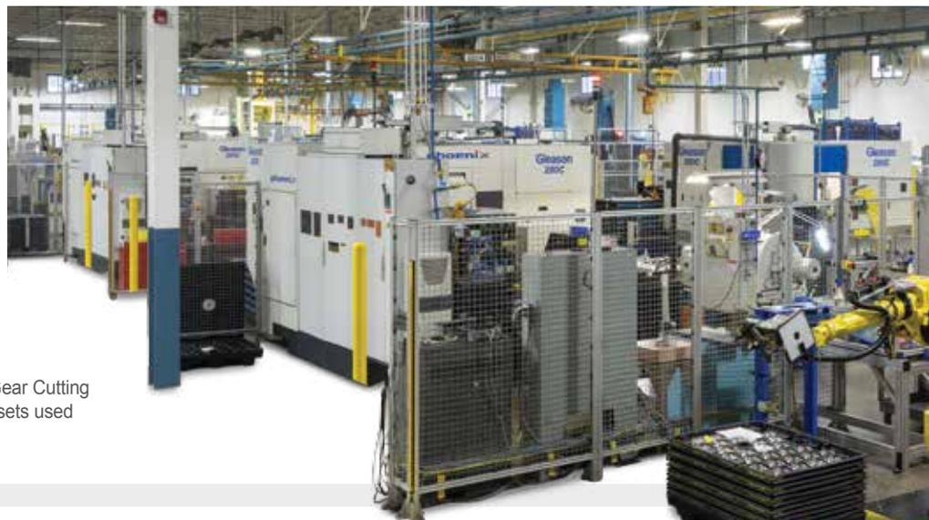
machine will be waiting a lot," Chandler says. "On the 280G, we use the robot to not only load and unload the machine, but also to hold the part for cleaning and pick and place the part at laser etching and palletizing."
