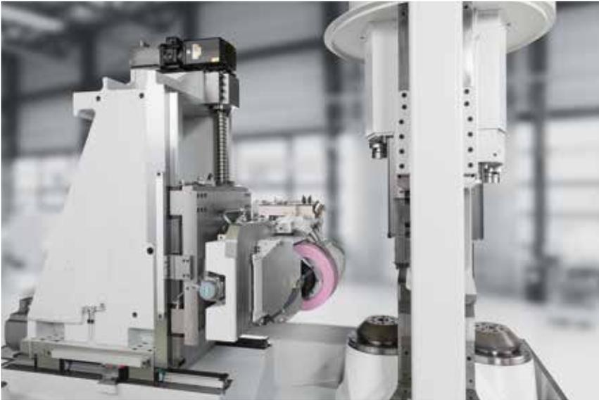
Double spindle concept for short idle times.
