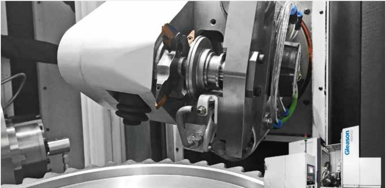
Chamfer contour milling employs a fly cutting process using milling cutters with indexable carbide inserts featuring two or four blades. A few insert sets can cover a wide range of modules making the fly cutting process extremely flexible while at the same time relatively inexpensive.
