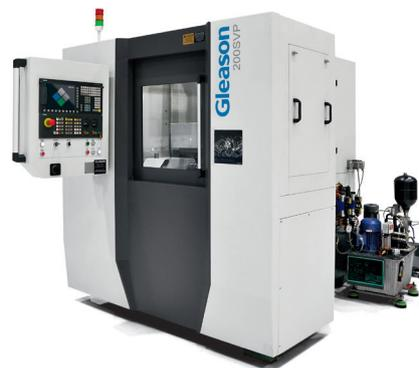
The new Gleason 200SVP is ideally suited for production of automotive gears and shafts using the economical plunge shaving process.
