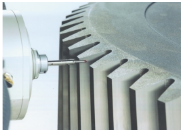
Fully automated gear inspection.
