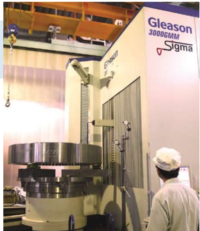
Two Gleason 3000GMM Analytical Gear Inspection Systems give Iwasa Tech the ability to meet stringent windpower quality needs.
