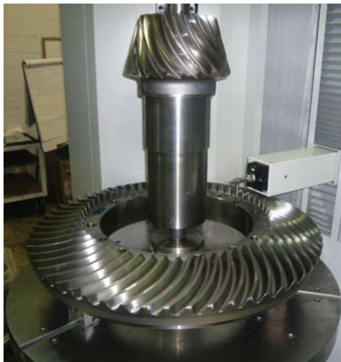
The Gleason 3000GMM's are versatile too, giving Iwasa Tech the means to inspect a complete range of products, including large bevel gears.
