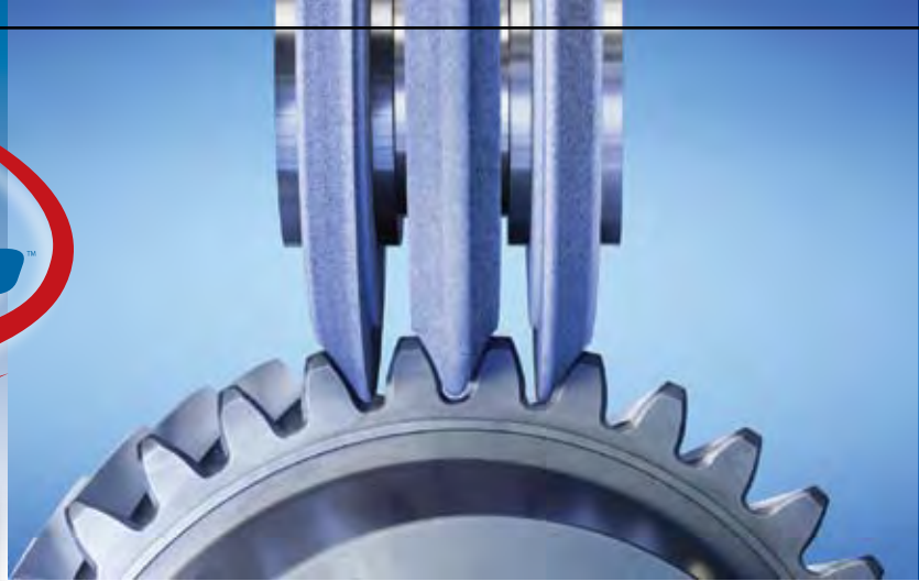
(Fig. 1) Maximum OPTI-GRIND productivity: an assembly of three dressable wheels rough grinds four tooth flanks simultaneously, as compared to typical use of a single wheel roughing two flanks at once. The center wheel only then is used for finishing, with desired surface finish and flank modifications dressed into the wheel.
