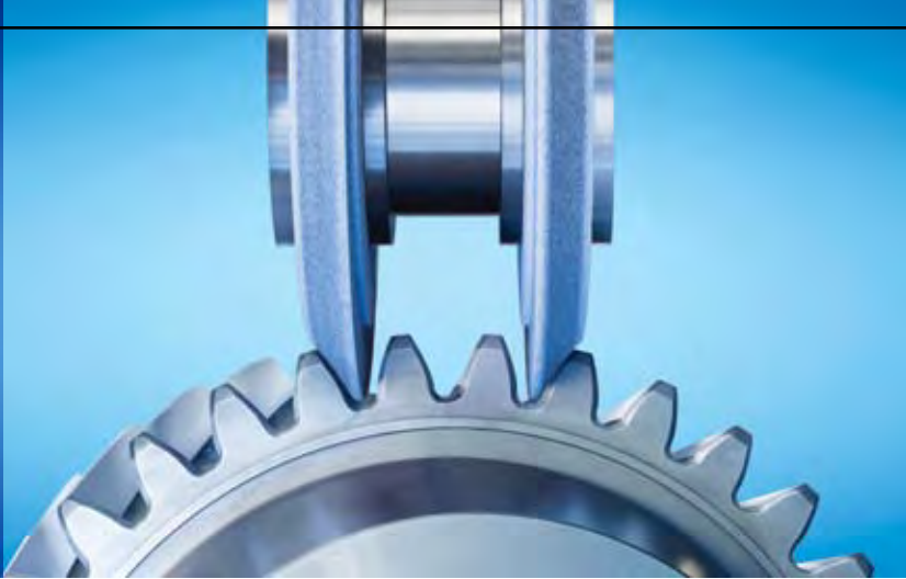
(Fig. 2) Ideal for pinion gear production: Another OPTI-GRIND variation shown here uses just the two outer wheels with each grinding a flank on separate gear teeth simultaneously. This variation reduces the radial infeed required as compared to grinding conventionally with a single wheel.
