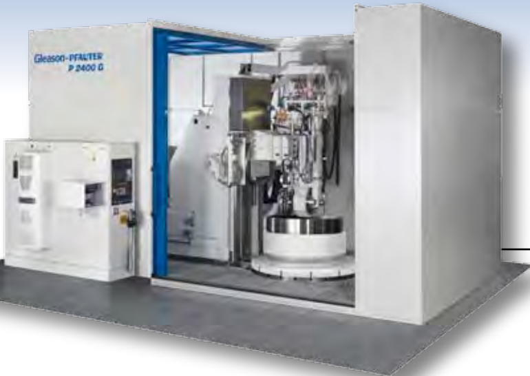
(Fig. 1) Maximum OPTI-GRIND productivity: an assembly of three dressable wheels rough grinds four tooth flanks simultaneously, as compared to typical use of a single wheel roughing two flanks at once. The center wheel only then is used for finishing, with desired surface finish and flank modifications dressed into the wheel.
