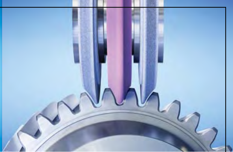
(Fig. 3) Maximum OPTI-GRIND surface finish quality: A third variation uses two outer wheels with an aggressive grit size to each rough grind a flank on separate gear teeth; then the middle wheel, shown here, with extremely fine grit size, finishes left and right flanks.
