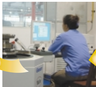
Gleason-Mahr GMX 600 Inspection System measures flank form errors...
