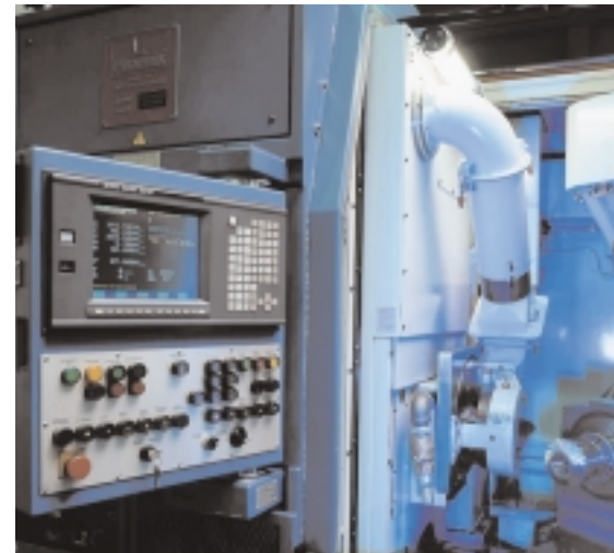
Gleason Phoenix® 175HC Power Cutting® Bevel Gear Cutting Machine performs soft cutting operations dry and with production rates many times faster than conventional methods.
