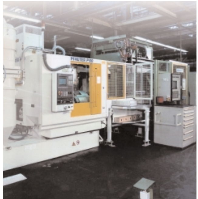
MITEC’s engine balancer systems use cylindrical gears produced on Gleason and Gleason-Pfauter gear cutting machines.
